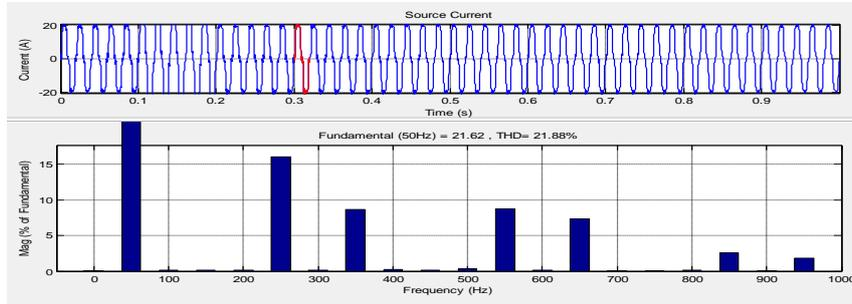
**Figure 22** Source current and Harmonic spectrum with Active Power filter
