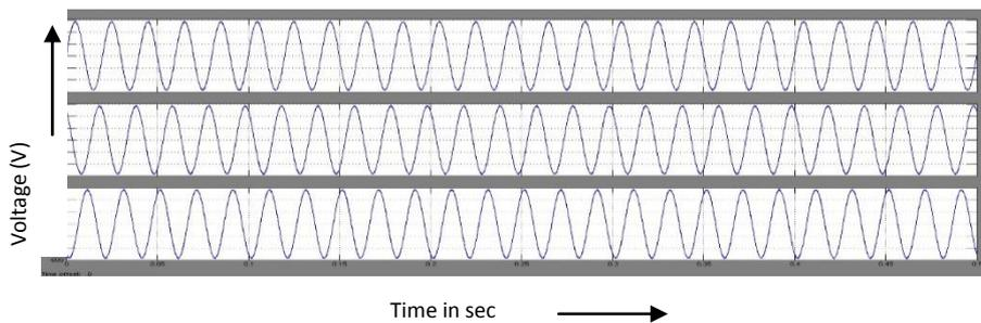
**Figure 21** Load voltage with DVR
