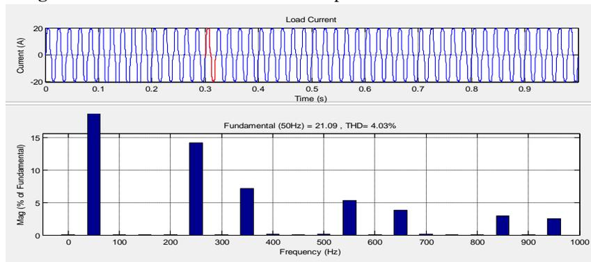
**Figure 23** Load current and Harmonic spectrum with Active filter
