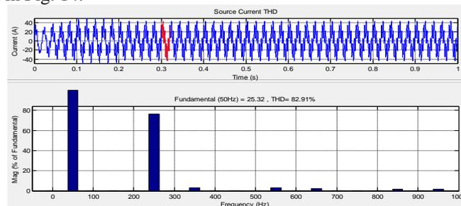
Figure 13 Source current and Harmonic spectrum with Active power filter
