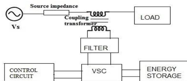
Figure 1 Block Diagram of DVR
