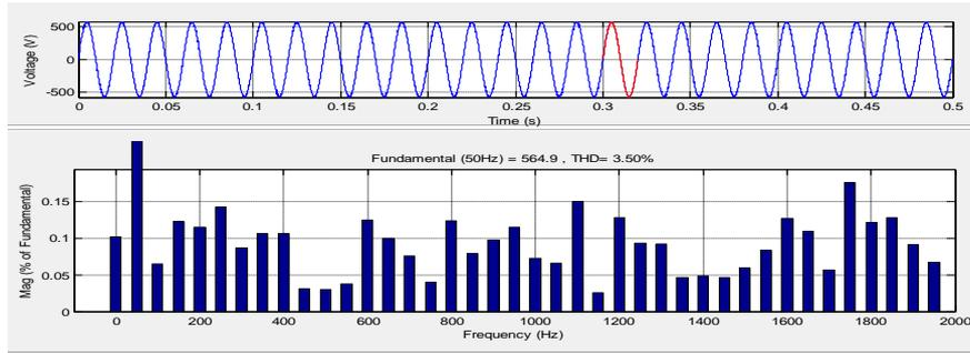
**Figure 18** Load voltage and harmonic spectrum with sag
