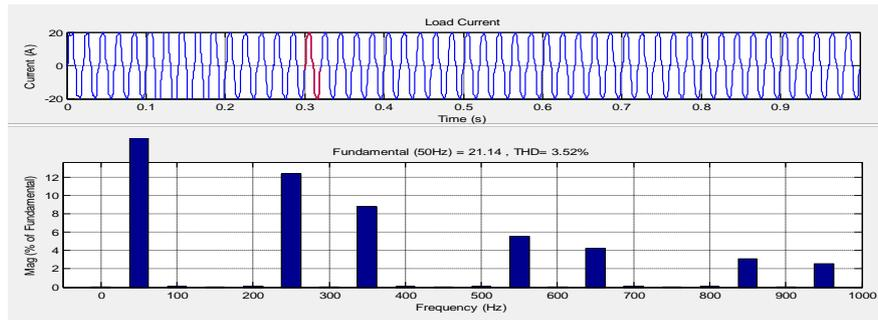
Figure 25 Load current and Harmonic spectrum with Hybrid Active Power filter
