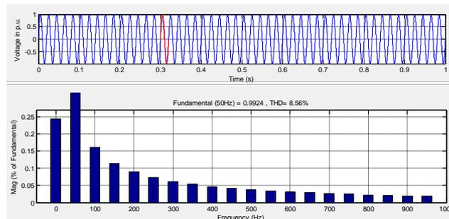
**Figure 10** Load Voltage and Harmonic spectrum with DVR
