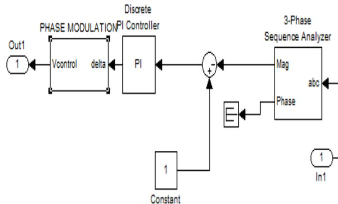
Figure 5 Control circuit
