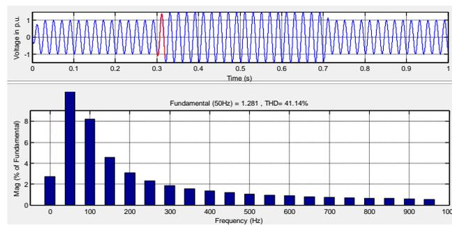
**Figure 9** Source Voltage and Harmonic spectrum with Swell
