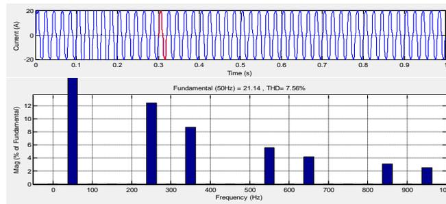
**Figure 16** Load current and Harmonic spectrum with Hybrid Active Power Filter
