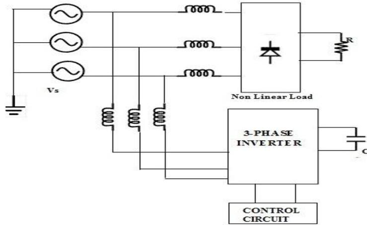
Figure 3 Three-phase Active Power Filter
