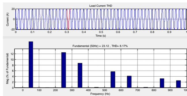
Figure 14 Load current and Harmonic spectrum with Active power filter
