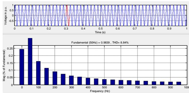
**Figure 8** Load Voltage and Harmonic spectrum with DVR
