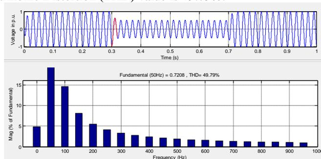
**Figure 7** Source voltage and Harmonic spectrum with voltage sag
