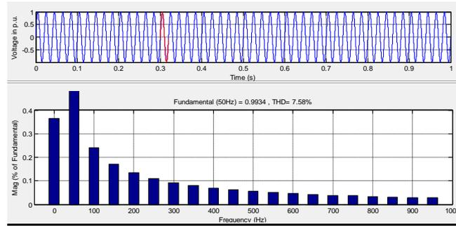
Figure 12 Load voltage and Harmonic spectrum with DVR
