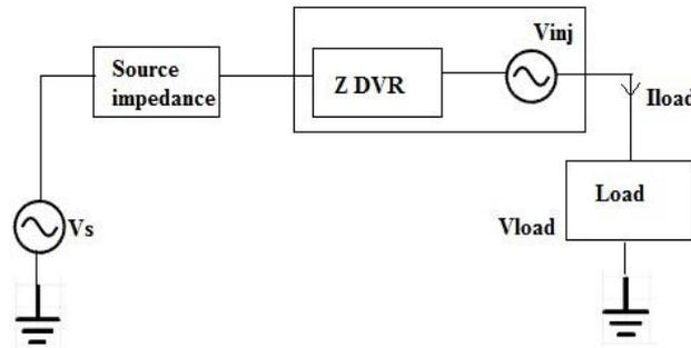
Figure 2 Equivalent circuit diagram of DVR
