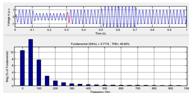
**Figure 11** Source Voltage and Harmonic spectrum with sag and swell
