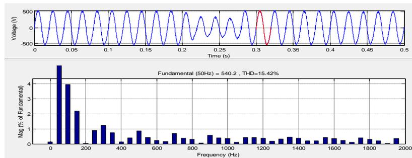
**Figure 17** Source voltage and harmonic spectrum with sag
