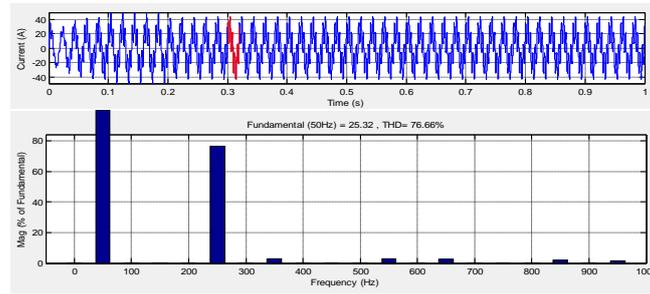
**Figure 15** Source current and Harmonic spectrum with Hybrid Active Power filter
