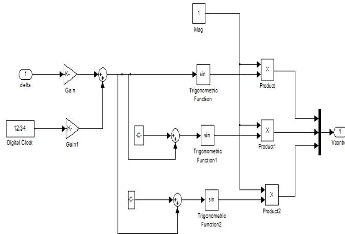
Figure 6 Phase modulation control circuit
